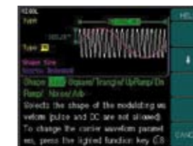
Built-In Help Easy access to the built in help system by pressing the key for 3 seconds.
