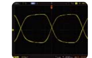
Rising and Falling Edge Triggering Mainly used to view eye-diagrams formally only available in more advanced DSO's.
