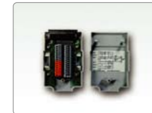
Internal View of Multiplexer Module
